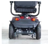
Rear bumper, indicators & anti-tip wheels
