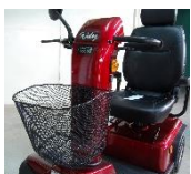
Hand brake, basket, two mirrors & indicators
