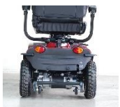
Rear bumper, indicators & anti-tip wheels
