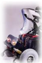
Lifting rear cover for quick maintenance
